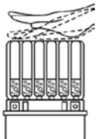
**2.1.5** Remove container and allow battery to stand for 20 minutes to allow the electrolyte to permeate into the plates.
