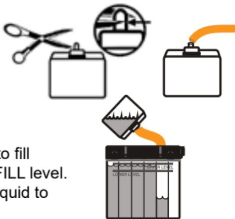
**2.2.4.** Tilt the electrolyte bottle to fill each individual cell to UPPER FILL level. Do not use water or any other liquid to activate the battery.
