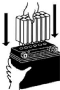
**2.1.4** Ensure electrolyte container completely empties. If no air bubbles are coming from the filler ports or if the container cells haven't emptied, tap the container a few times. Please do not remove the electrolyte container until it is empty.
