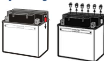
**2.2.2.** Remove filling plugs located on battery top. And connect transparent exhaust pipe to the battery exhaust nozzle.
