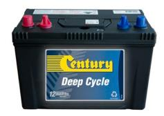
Century Deep Cycle Flooded batteries are constructed using thicker plates, specialist lead calcium alloys and denser active material, to withstand repeated recharge and discharge cycles. Premium grade raw materials and electrolyte ensures reliable deep cycle performance in recreational applications.
